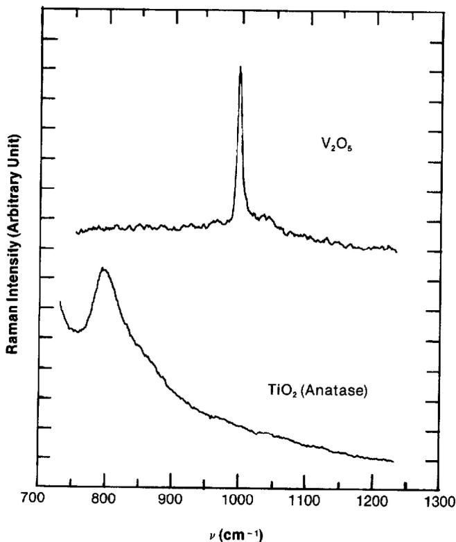
Figure 2 Laser Raman Spectra of Unsupported V<sub>2</sub>O<sub>5</sub> and TiO<sub>2</sub>(Anatase).
