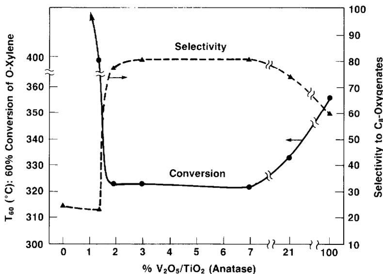
Figure 6 O-Xylene Activity and Selectivity Towards  $C_8$ -Oxygenates Over Unsupported  $V_2O_5$  and  $V_2O_5/TiO_2$ (Anatase) Catalysts.
