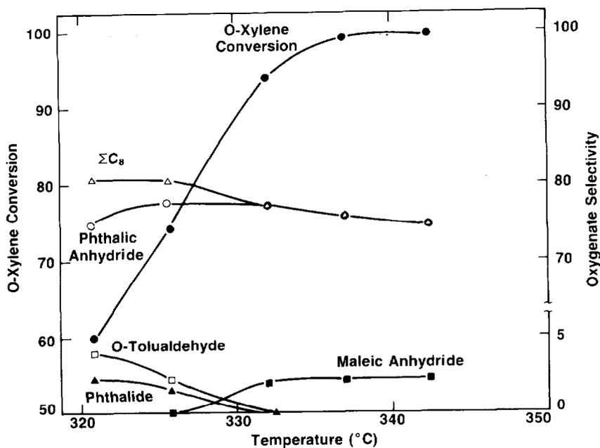
Figure 5 Conversion of O-Xylene and Selectivity Towards Various Oxidation Products as a Function of Catalyst Temperature for the 7% V<sub>2</sub>O<sub>5</sub>/TiO<sub>2</sub>(Anatase) Sample.
