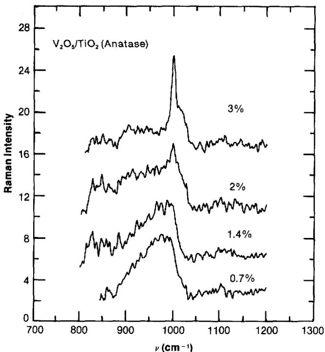
Figure 3 Laser Raman Spectra of Low Surface Area  $V_2O_5/TiO_2$ (Anatase) as a Function of  $V_2O_5$  Content (all spectra corrected for  $TiO_2$ (anatase) background).
