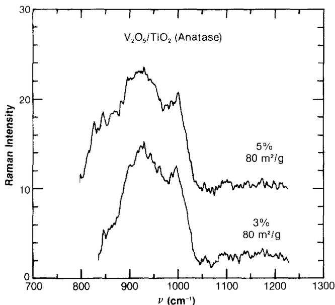
Figure 4 Laser Raman Spectra of High Surface Area  $\text{V}_2\text{O}_5/\text{TiO}_2(\text{Anatase})$  as a Function of  $\text{V}_2\text{O}_5$  Content (all spectra corrected for  $\text{TiO}_2(\text{anatase})$  background).
