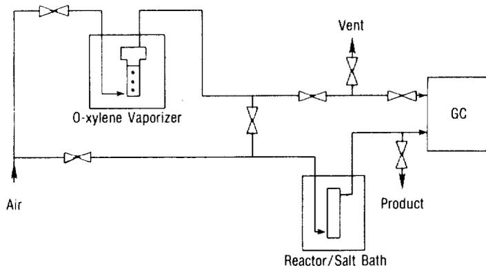
Figure 1 Schematic of Reactor Unit for the Oxidation of O-Xylene to Phthalic Anhydride.
